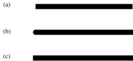
Figure 9.2: Cap styles: (a) butt, (b) round, (c) square. Note that the round and square caps protude from the start and end vertices.
