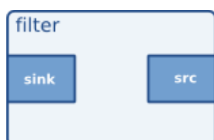
Figure 5-2. Visualisation of a filter element
