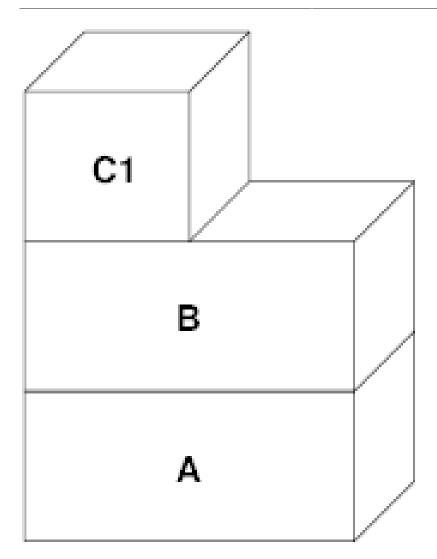
In this case, the number of children of B drops to one, and all accesses to B now go through C1. This means that B and C1 can be collapsed together. Any pages in B that also exist in C1 are deleted from B during the collapse. Thus, even though the optimization in the previous step could not be made, we can recover the dead pages when either of the processes exit or exec().
